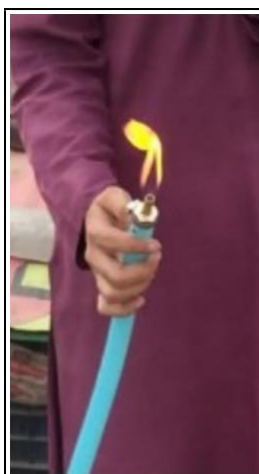
Figure 4: Live flammability check of the non-condensable gas at the exhaust point.
