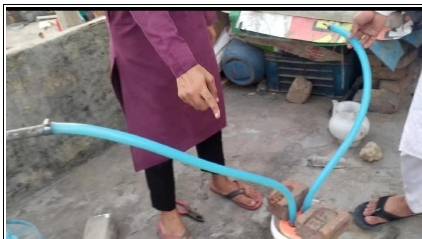
Figure 2: Custom water-cooled condensation pipe arrangement used in our experiment.
