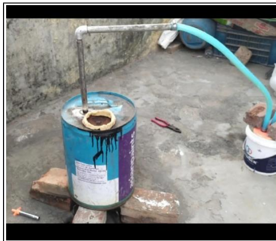
Figure 1: Simple fabricated batch reactor setup built on brick foundation.
